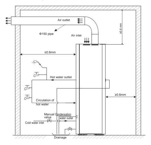
The minimum permissible distances to adjacent structures: In order to the air flow will not be affected, please make sure the distance that between the top of units and ceiling specific parameters.
